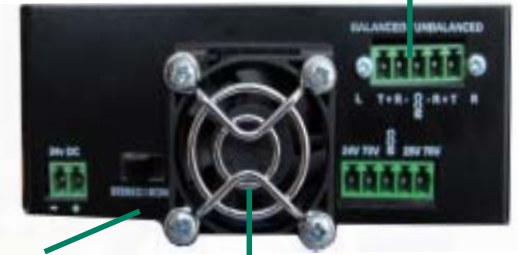
AUTOMATIC FAN CONTROL FAN TURNS OFF AUTOMATICALLY WHEN NO AUDIO IS PRESENT
